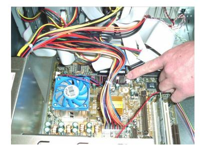
A. Insert 1GB of RAM into the slots closest to CPU
