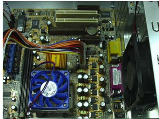
**D. Get network card and place in first PCI slot from power supply**
