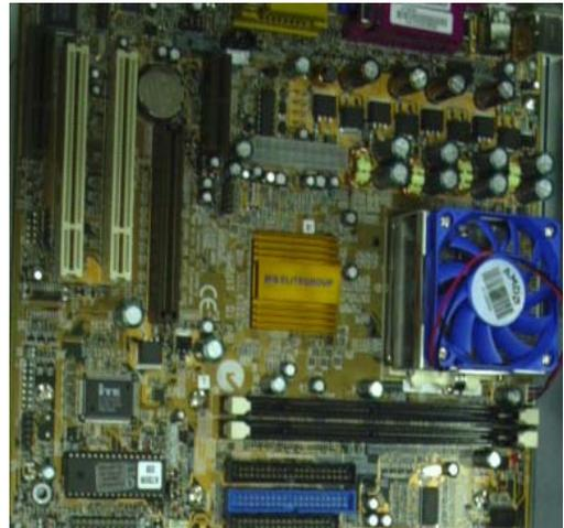
**L. Connect CPU fan to motherboard**
