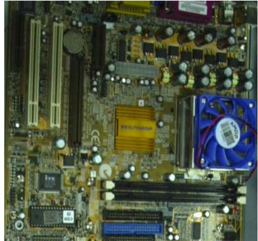
**L. Connect CPU fan to motherboard**
