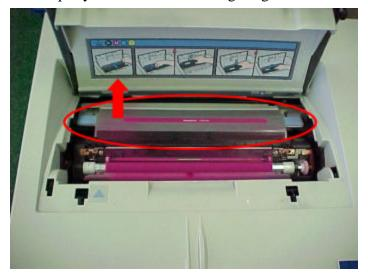
iv. Lift up the panel circled in the picture, in the direction indicated by the arrow
